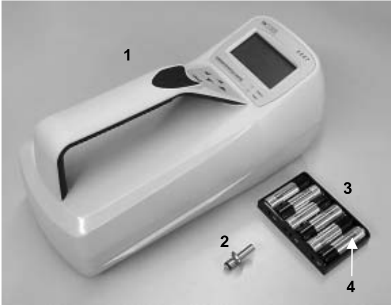
Figure 1-1: Model 3007 Condensation Particle Counter With Inlet Probe Assembly, Battery Pack, and Batteries
