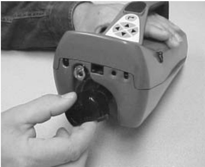
Figure 2-6: Insert Alcohol Cartridge into Condensation Particle Counter
