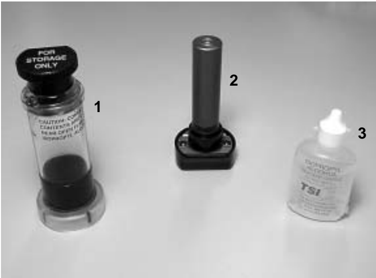
Figure 1-2: Alcohol Fill Capsule with Storage Cap, Alcohol Cartridge, Alcohol Bottles and Shoulder Strap
